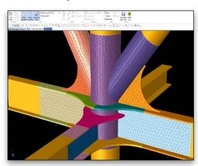
Graphical user interface for the design and automatic meshing of stiffened nontubular joints.
