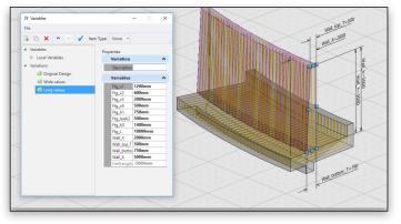
ProConcrete delivers a feature called faced-based rebar modeling, allowing users to add 3D steel reinforcing bars that are parametric to concrete faces. This enables changes to the concrete faces to automatically correct the rebar.
