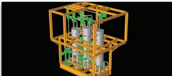
SACS – Combined piping and structural model (secondary steel in green)
